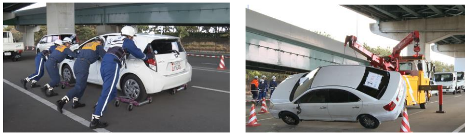
Figure 7 Moving out Stalled Vehicles using a GOJAK, a vehicle lifting and carrying dolly or a wrecker.
