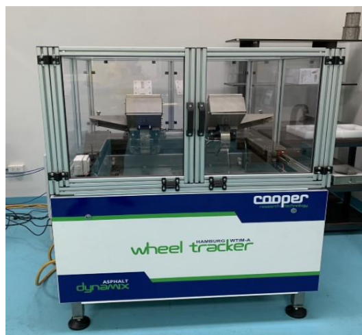
Figure 10: Hamburg Wheel-Tracking (Department of Highways (Thailand))
