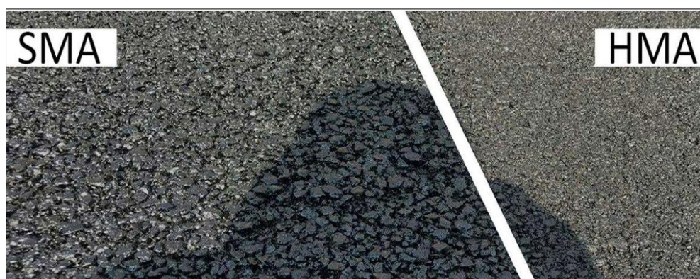
Figure 2 : Physical characteristics of SMA vs Conventional Mix Asphalt
