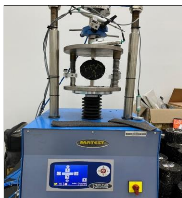
Figure 6: Indirect Tensile Strength Apparatus
